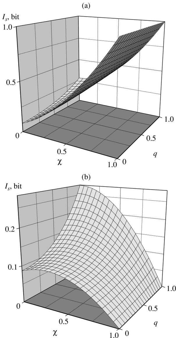
**Fig. 7.** Selected information  $I_s$  in a two-qubit system vs. degree of selectivity  $\chi$  and entanglement parameter  $q$  for the (a) parallel ( $\vartheta = 0$ ) and (b) crossed ( $\vartheta = \pi/2$ ) orientations of selective measurements.
