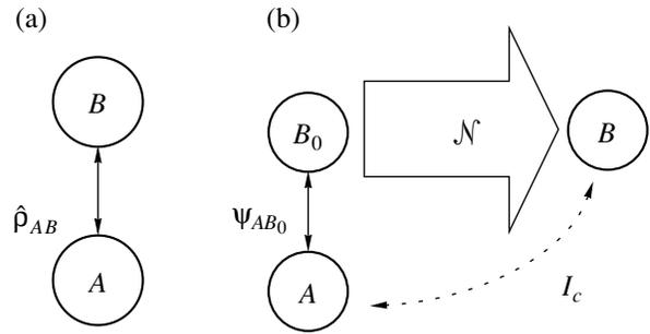
**Fig. 3.** Reconstruction of a quantum information system corresponding to given joint density matrix  $\hat{\rho}_{AB}$ : (a) mathematical description of the channel specifying one-time information and (b) its correspondence with the Schumacher construction [33].
