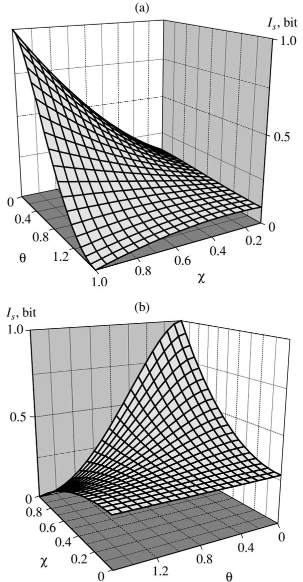
**Fig. 6.** Selected information  $I_s$  in a two-qubit system vs. degree of selectivity  $\chi$  and relative orientation of selective measurements  $\vartheta$  (a) in the absence of entanglement for quasi-classical information communication ( $q = 0$ ) and (b) for a pure entangled state ( $q = 1$ ).
