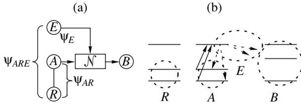
**Fig. 2.** (a) Block diagram of a quantum information system and (b) its possible physical realization: (A) input, (B) output, (R) reference system, and ( $\mathcal{N}$ ) channel with noisy environment  $E$ .
